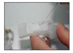
Put some glue on the chip position of CISS cartridge.
